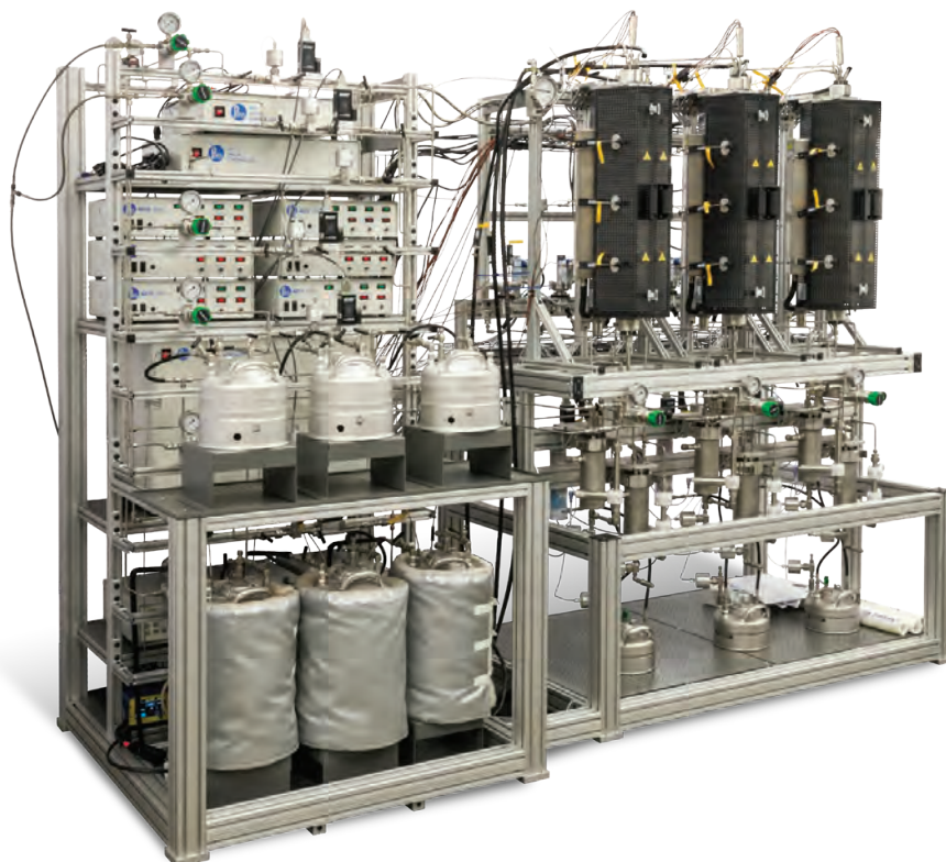
The system above has three 250 mL tubular reactors operating in parallel and controlled by a 4871 Process Controller with operator interface on a single PC. This system has weighed and/or heated feed tanks and a two-stage pressure let down.
