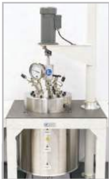
5 Gallon Stirred Vessel in stand with stirrer engaged.
