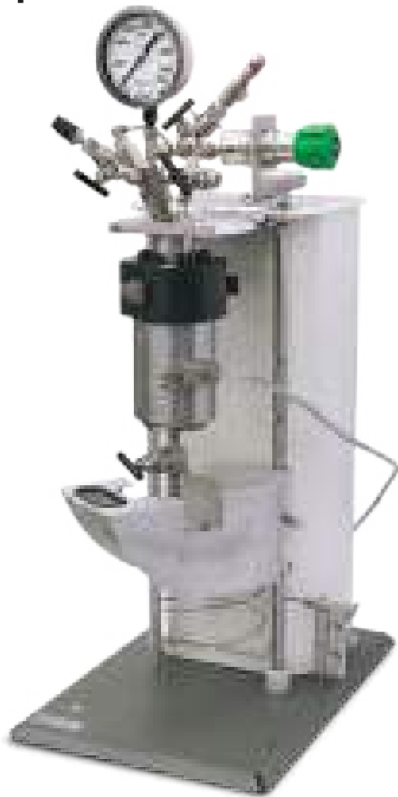
The batch supercritical water extraction vessel pictured above is constructed of Hastelloy C-276 and is designed for use to 6000 psi (410 bar) at 400 °C.
