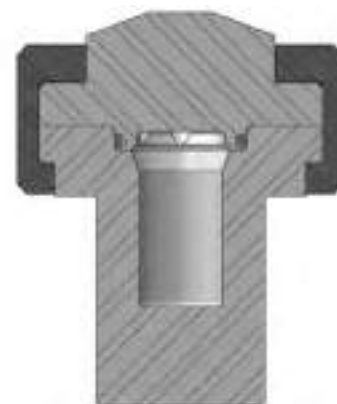
4790-25mL Cross Section with O-ring Seal
