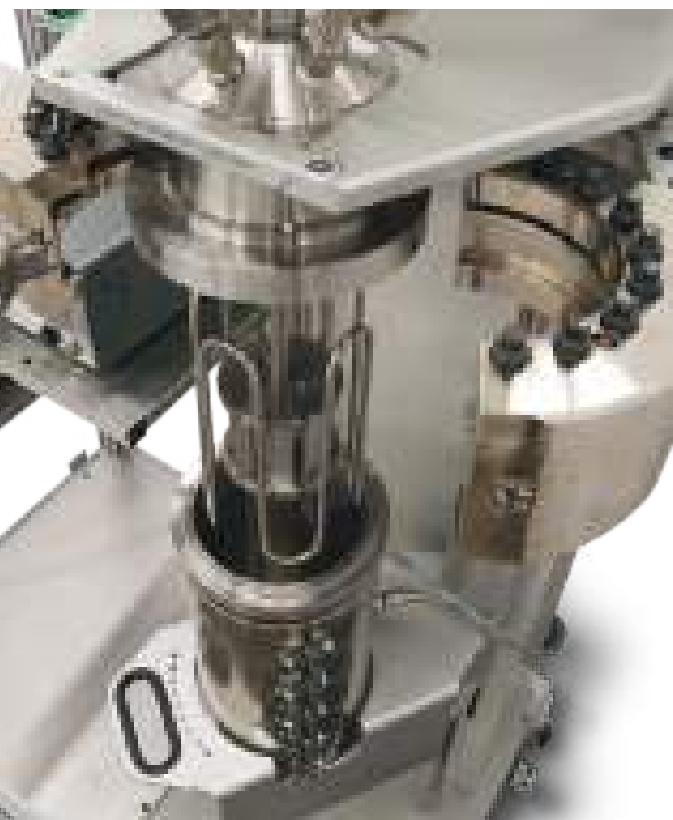
5 Liter Vessel lowered to reveal the rotating cage. In this configuration, up to 8 coupons at up to 2,000 rpm, can be tested at one time.
