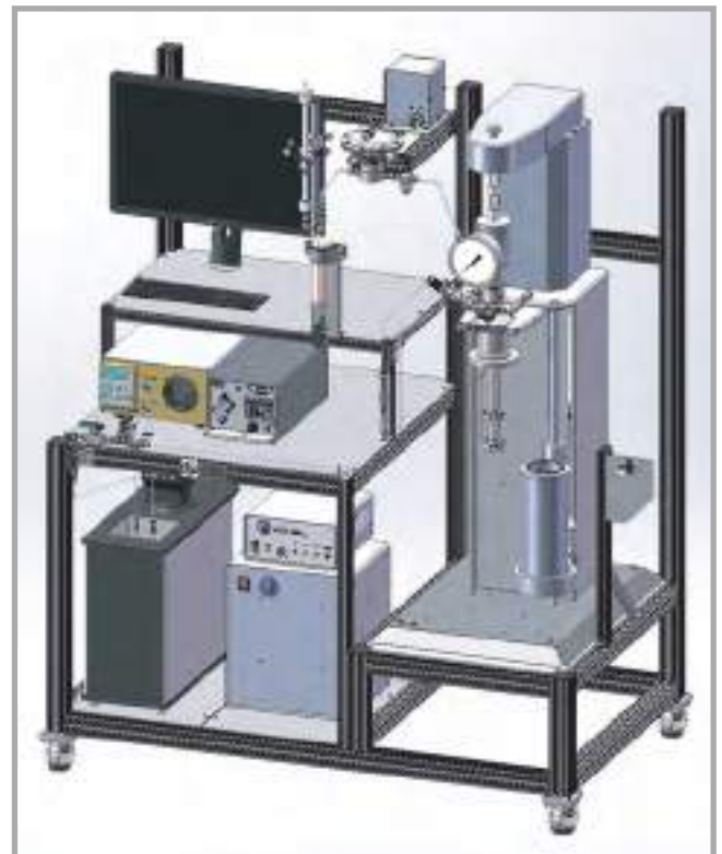
This batch carbon dioxide extraction system modelled above includes a 1.2 L extraction vessel rated to 5000 psi (345 bar), both CO 2 and co-solvent pumps, automatic pressure control and collection vessel with manual ball valve for extract collection, as well as custom control and data logging system with pre-programmed recipe list.
