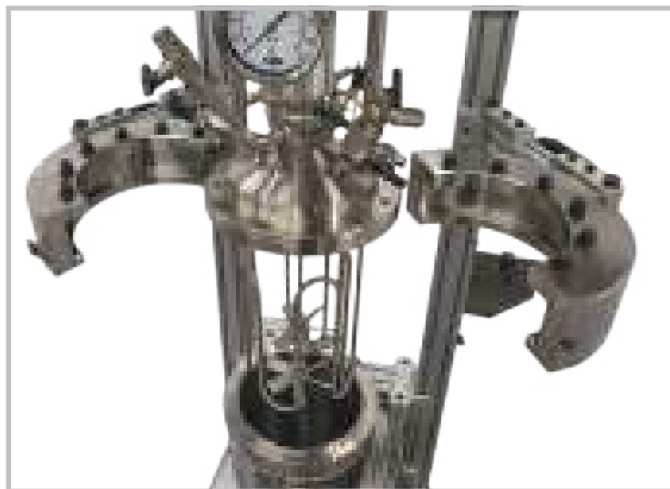
Hinged Split-Rings open to reveal Serpentine Cooling Coil, with Heater and Vessel lowered via Pneumatic Lift.
