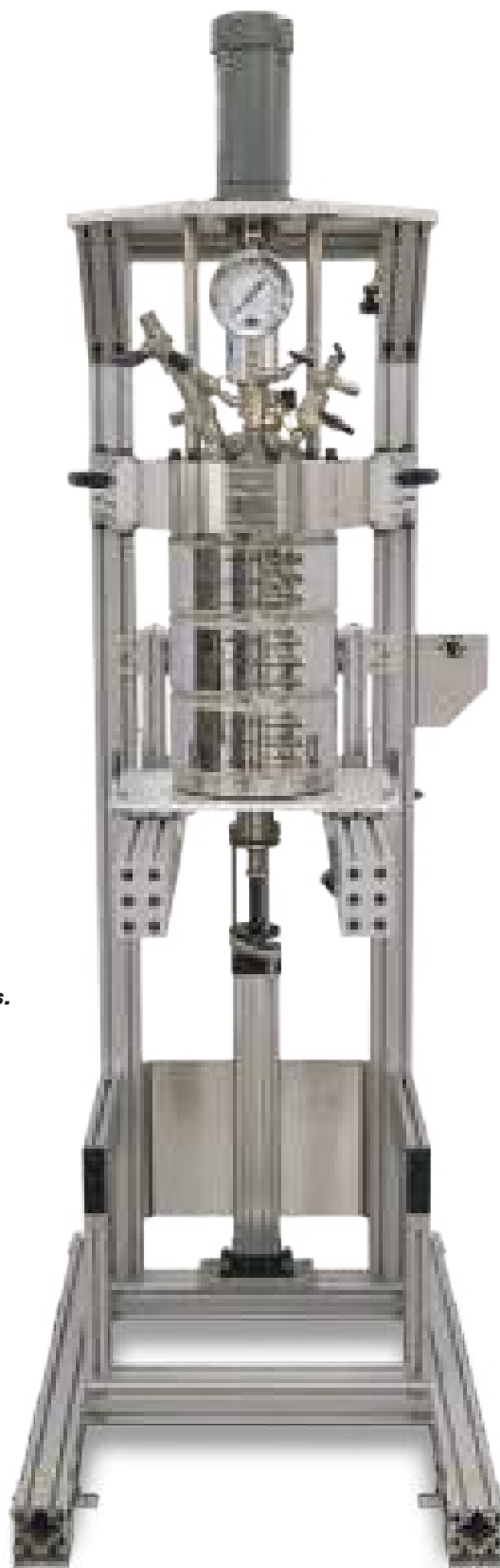
4557 Floor Stand Reactor, 5 Gallon, Fixed Head, 3-zone Band Heater, with Split-Rings and Pneumatic Lift.
