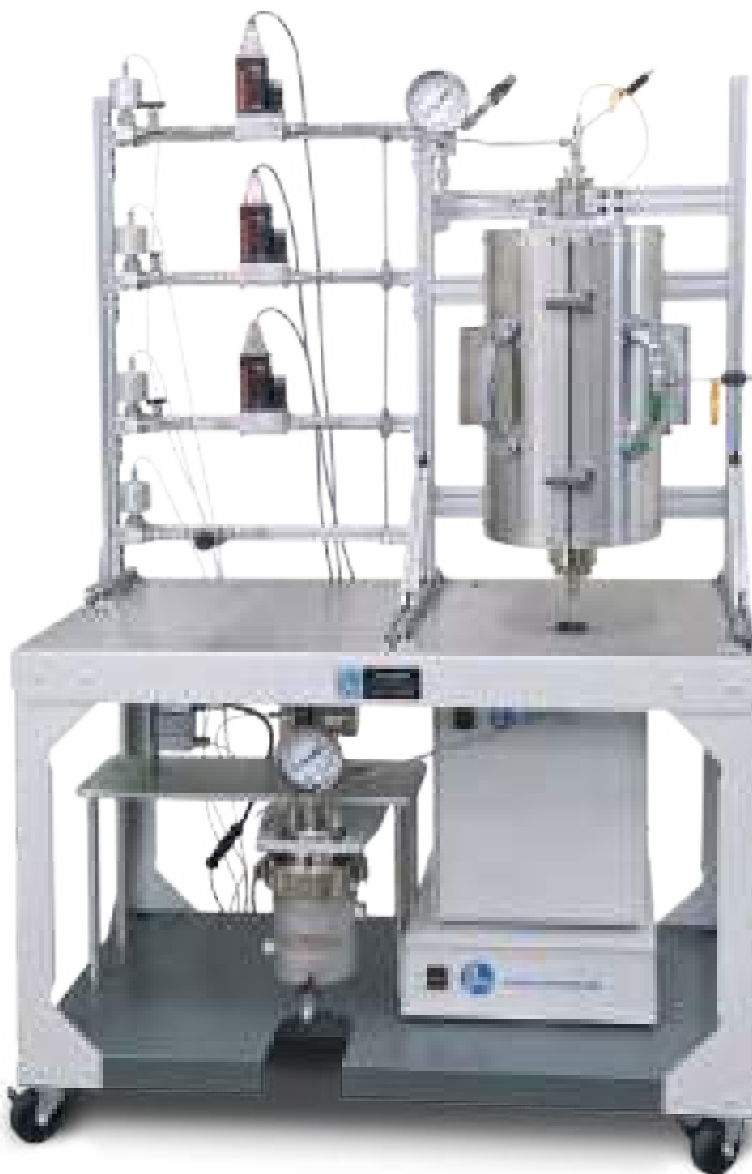
This tubular reactor system features a single-zone 12-inch long heater to take reactor temperatures to 500 °C. The gas feed system includes automated shut-off valves on the three MFCs and on the purge line. The Gas/Liquid Separator vessel is jacketed to allow for subambient cooling. Operator controls the system via a remote PC using the included Model 4871 Process Controller.
