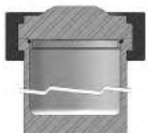
4660Q Cross Section with O-ring Seal
